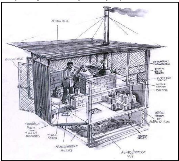
Figure 4: Components of a Waste Disposal Site incorporating the DeMontfort Incinerator
